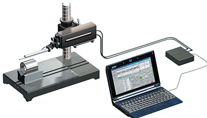
Fig. 1. MarSurf PS 10 MAHR needle profilometer
