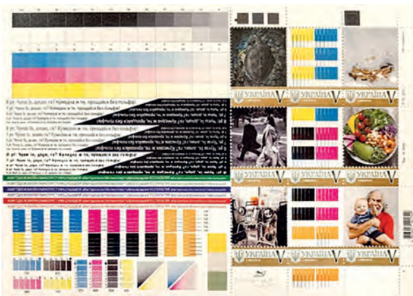
Fig. 4. Imprint on Mimaki UJF-3042FX digital printing machine (UV jet printing)
