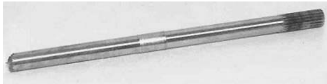
Fig. 9. External type of destroyed reducer shaft
