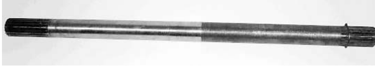
Fig. 1. Design of real input shaft from the reducer about rope electric hoist
